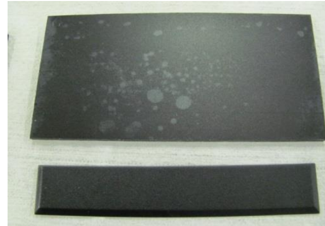
Coating 1 coated with insufficient UV energy
