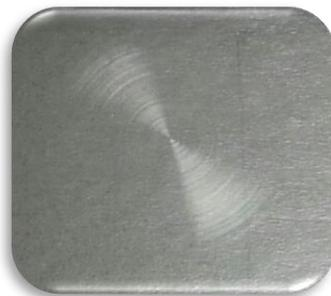
Figure 2 - Worn Rotary Steel Wool tested samples
