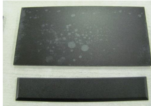
Coating 1 coated with insufficient UV energy
